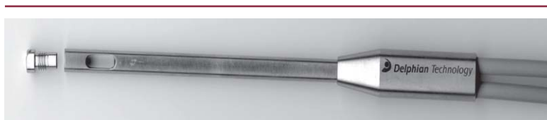
Figure 2: Fiber optic dip probe showing removable tip (20 mm path length)
