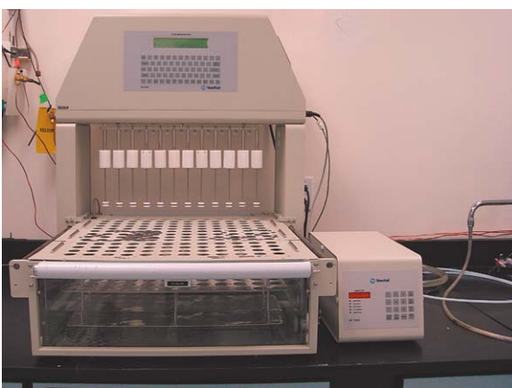
Figure 1. USP Apparatus 7 and the temperature controller (VK 750D Heater/Circulator) made by VanKel/Varian.
