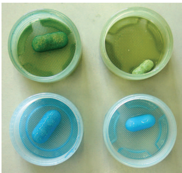
Figure 8. Contiphyllin 300-mg (left-hand side) and Tromphyllin retard 300-mg tablets (right-hand side) before and after a test duration of 4 h in compendial media (bottom) and Ensure Plus (top).
