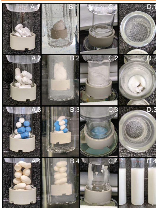
Figure 4. Photographs of 10 doses of acetaminophen during USP apparatus 3 testing. Row 1 shows IR tablets, 2 shows ER tablets, 3 shows hard capsules, and 4 shows soft capsules. A.1–A.4 depicts the dosage forms in the inner cylinder shortly before test start; B.1–B.4 is within first 2 minutes in FaSSGF; C.1–C.3 is after 60 minutes in FaSSGF, C.4 shows 10 soft capsules after 15 minutes in FaSSGF; D.1–D.3 shows inner cylinder content after finishing the test, and D.4 shows strongly colored FaSSGF buffer due to penetration of all soft capsule residuals into the outer vessel. USP: United States Pharmacopoeia; IR: immediate release; ER: extended release; FaSSGF: fasted state simulated gastric fluid.
