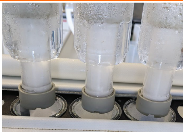
Figure 6. Photograph of 50 IR tablets after 60 minutes in FaSSGF buffer in USP apparatus 3. Clumped tablet material filled nearly the entire volume of the inner cylinder. This was observed in all five compartments (up to 6 hours).
